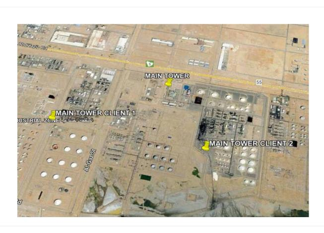
At "MAIN TOWER" point of presence we've got two radios, one pointing to the east, 275 degrees, and the other to the south, 180 degrees.
